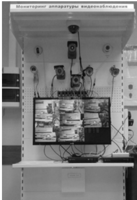
Fig. 1. Stand organization monitoring surveillance equipment
